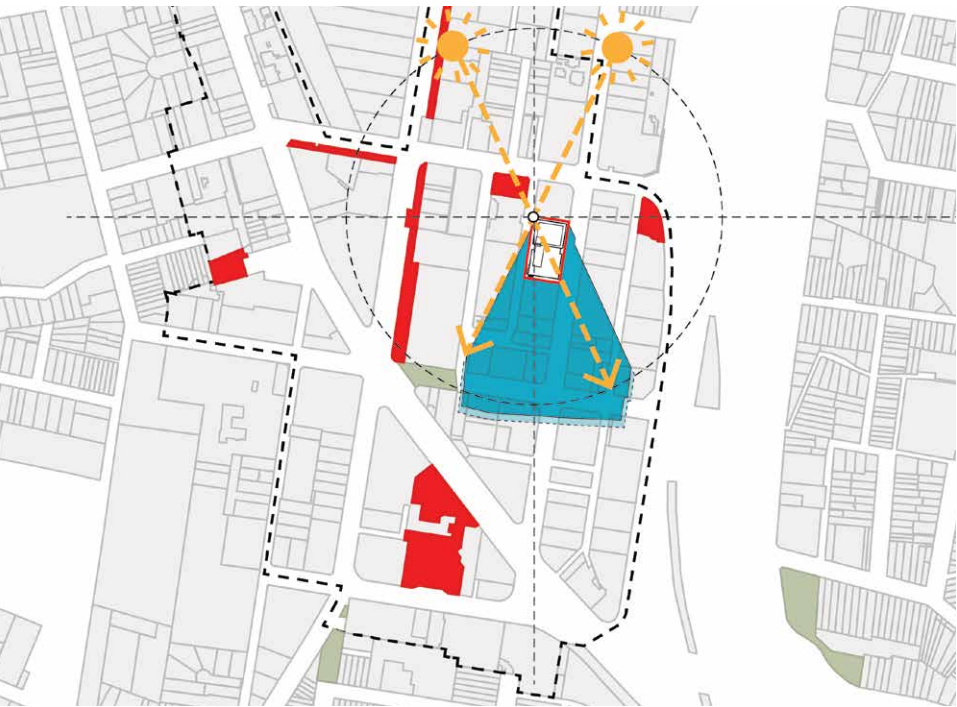
Autumn Equinox 12:00 PM Solar Azimuth Angle 26.4° Altitude 52.8° 2:00 PM Solar Azimuth Angle 335.4° Altitude 53.2°
