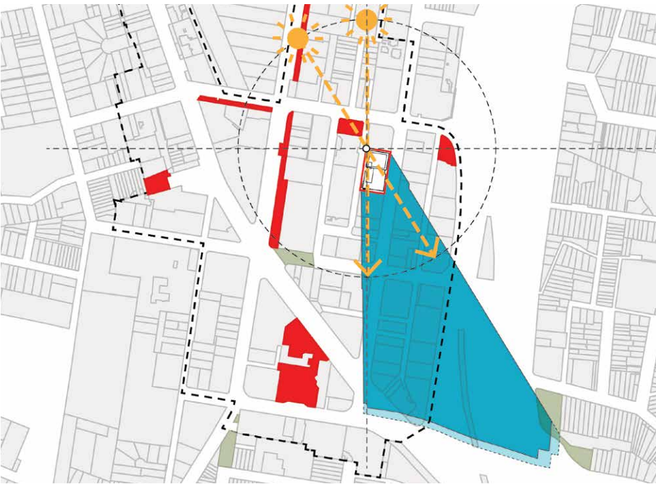
Winter Solstice 12:00 PM Solar Azimuth Angle 359.2° Altitude 32.7° 2:00 PM Solar Azimuth Angle 328.6° Altitude 25.7°
