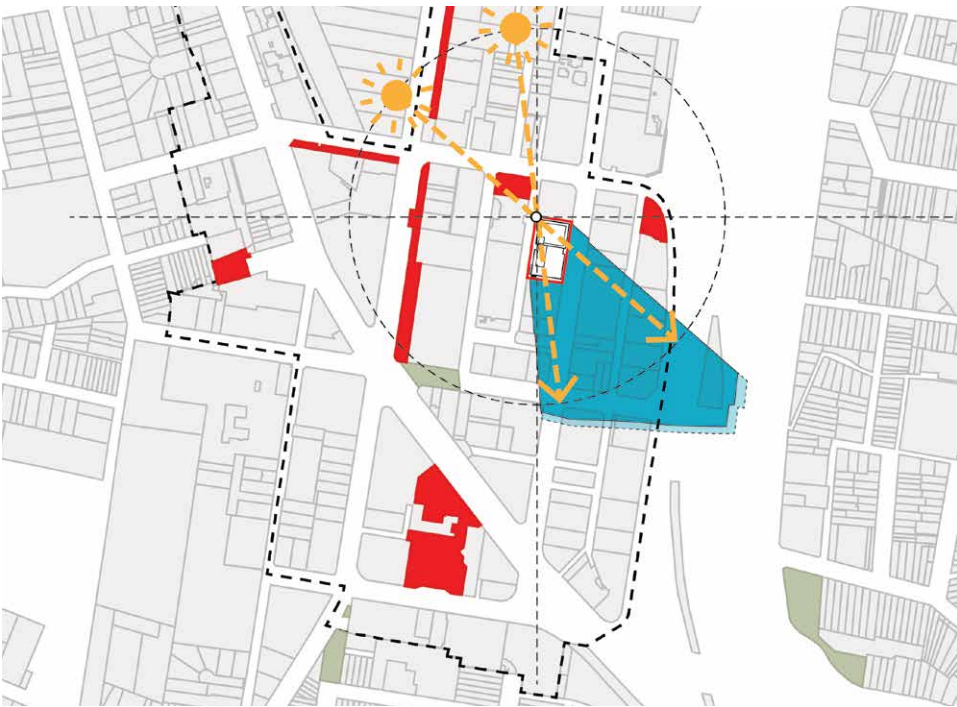
Spring Equinox 12:00 PM Solar Azimuth Angle 354.8° Altitude 55.5° 2:00 PM Solar Azimuth Angle 311.1° Altitude 43.8°
